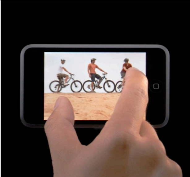
To zoom in on a picture, users take advantage of the 'Pinching' technique.
